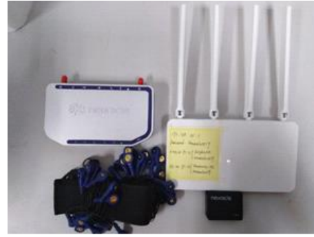
Figure 2. Surface EMG signal acquisition device utilizes. NeuroCube-NSW308 surface EMG signal acquisition instrument manufactured by Neuracle company, Wi-Fi module.
